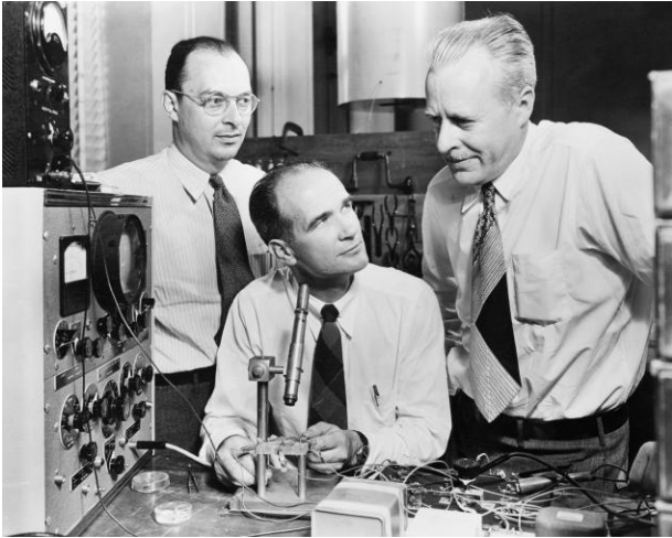
Shockley studying the apparatus used by Bardeen (left) and Brattain (right) to demonstrate transistor amplification. [Bell Labs photo]
